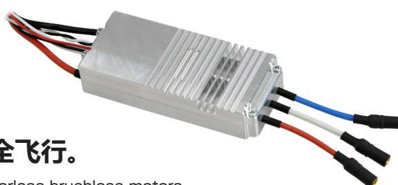
An electronic speed controller (ESC) dedicated to sensorless brushless motors.
